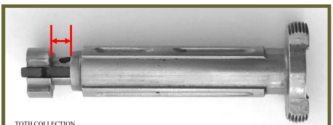
Top: Bolt showing one of the helix grooves. Lower left: Bolt carrier showing internal studs that engage the helix grooves of the bolt. Lower right: Bolt inserted into bolt carrier until lugs of both are aligned. (Lower right image is upside down from normal position when installed).
