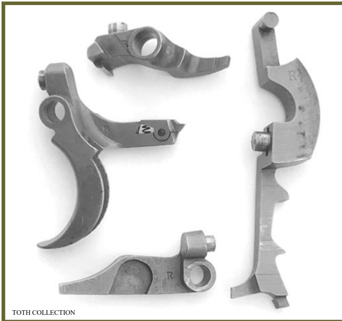
Note the capital "R" on the small parts (as well as more captured springs).
