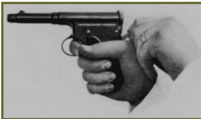
De-cocking with two hands (from a French language Frommer pistol manual).
